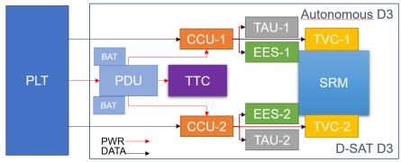
CDF ESA CleanSat Technology Assessment: Building Block 14 - Autonomous De-Orbit System
